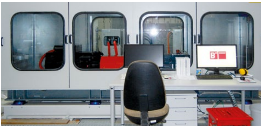
Test stand for electrical machines and engines: Focus on electromobility and energy efficiency
