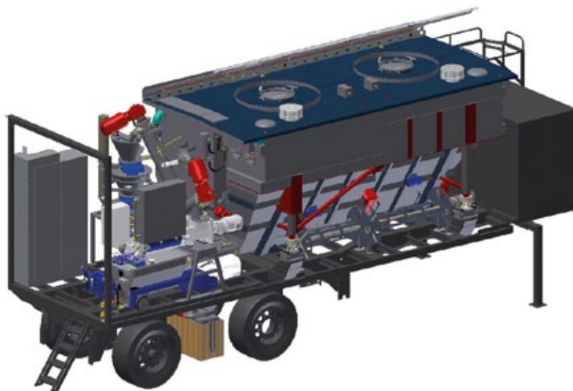
Mobile PumpTruck m-tec PT equipped with Berghof control technology
